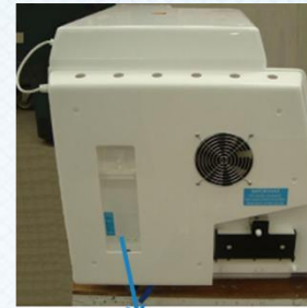
Pressure Relief Tank
